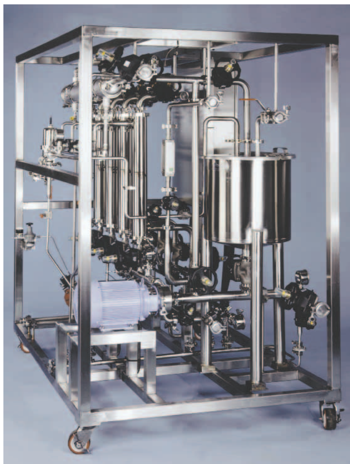
Figure 42. Custom engineered system with Steam-in-place capability
