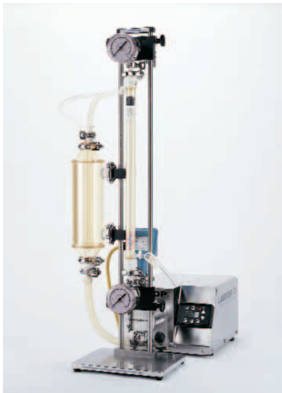
Figure 36. Low void volume FlexStand system
