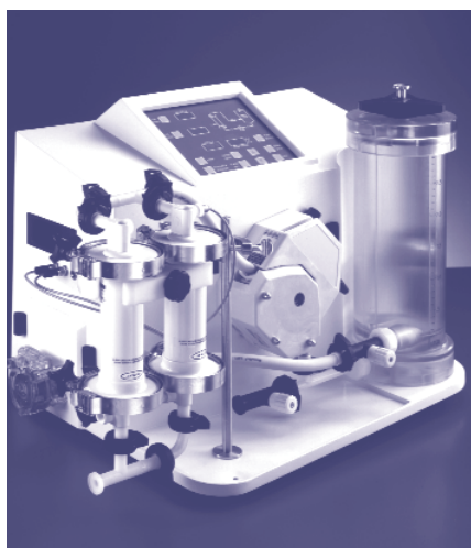
ProFlux® M12 Benchtop TFF system with spiral wound modules
