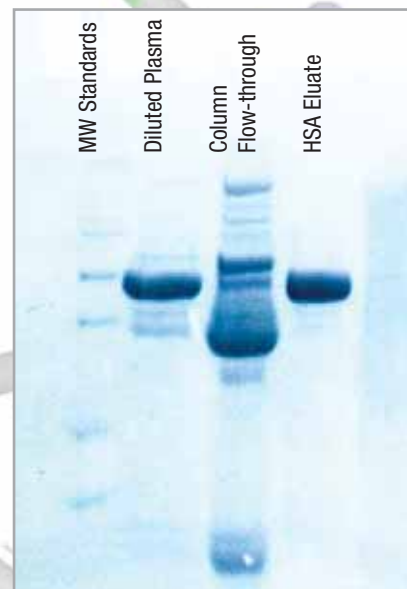
Purification of HSA from plasma using Mimetic Blue SA
