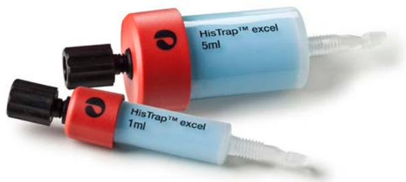
Fig 3.32. HisTrap excel allows direct purification of cell-free, unclarified samples; it is available as 1 ml and 5 ml preppacked columns.
