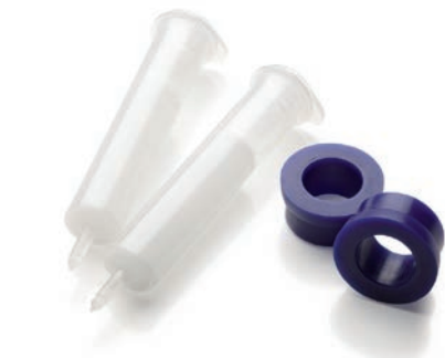
Fig 2.13. PD MidiTrap G-25 is a prepacked column for cleanup of proteins with a molecular weight > 5000 in sample volumes up to 1 ml.
