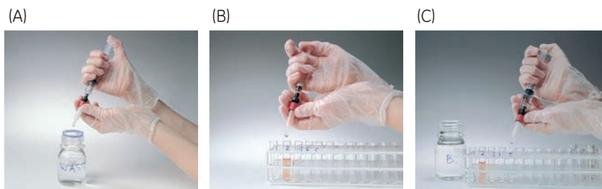
Fig A4.1. Using HiTrap columns with a syringe. (A) Prepare buffers and sample. Remove the column's top cap and twist off the end. (B) Equilibrate the column, load the sample and begin collecting fractions. (C) Wash and elute, continuing to collect fractions.
