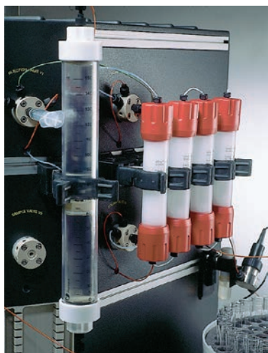
Fig 2.6. A 60 ml sample volume can be run on four HiPrep 26/10 Desalting columns connected in series.
