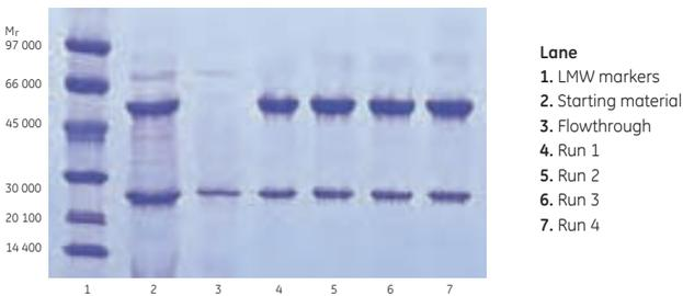
**Fig 6.9.** SDS-PAGE purity analysis (reducing conditions) of human monoclonal antibody purified by affinity chromatography using ÄKTExpress. Lanes 4–7 are fractions from the final desalting steps shown in Figure 6.8. Data kindly provided by G.J. Perdock, T. Verhagen and P.H.C. van Berkel, Genmab BV, Utrecht, Netherlands, and used with permission.
