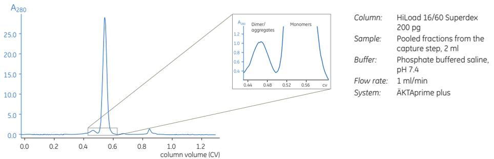
**Fig 6.6.** Note the separation between dimers and monomers (magnified).
