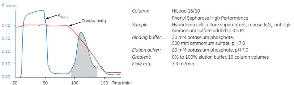
Fig 6.10. Capture of mouse IgG<sub>1</sub> on HiLoad 16/10 Phenyl Sepharose High Performance.
