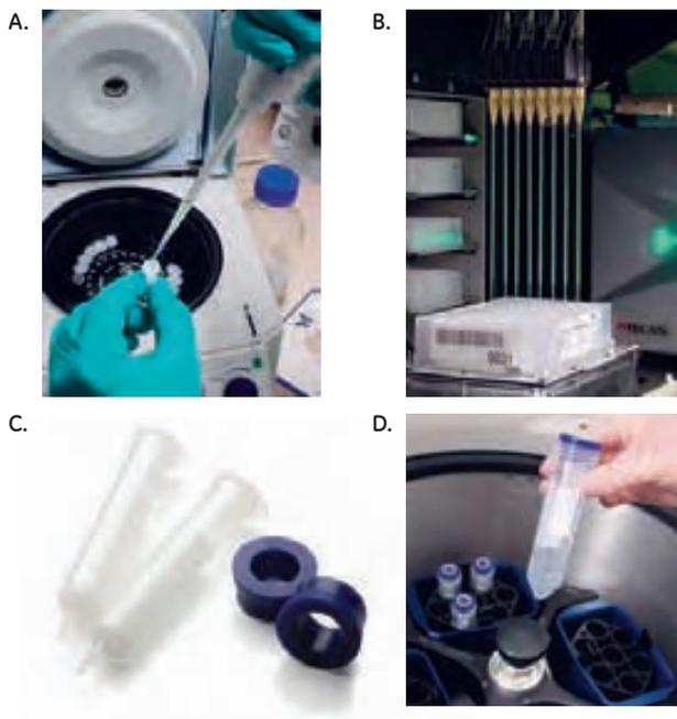
**Fig 2.2.** (A) PD SpinTrap G-25 sample preparation. (B) PD MultiTrap G-25 sample automated preparation in a robotic system. (C and D) Spin Adapters are used together with PD-10 Desalting Columns, PD MidiTrap G-25, and PD MiniTrap G-25 to enable use in a standard centrifuge.
