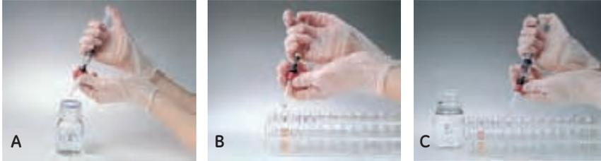
**Fig A4.1.** Using HiTrap columns with a syringe. **(A)** Prepare buffers and sample. Remove the column's top cap and twist off the end. **(B)** Equilibrate the column, load the sample and begin collecting fractions. **(C)** Wash and elute, continuing to collect fractions.
