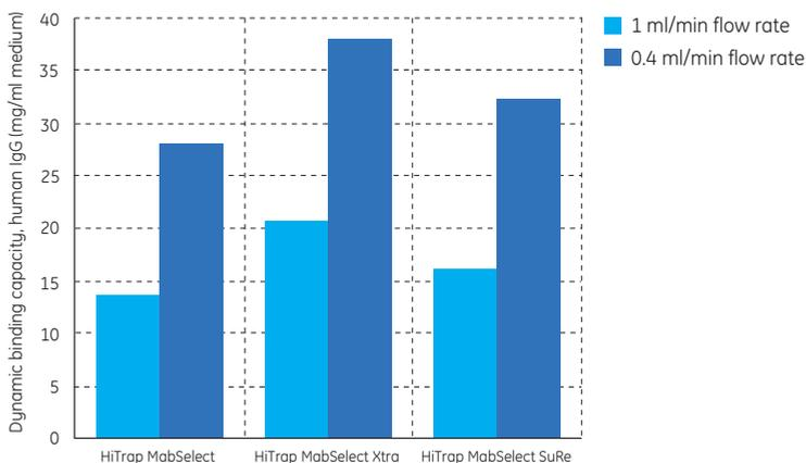
**Fig 3.23.** MabSelect media feature a highly cross-linked agarose, produced using a manufacturing process that gives a very rigid matrix that is optimal for high-throughput affinity chromatography of IgG.
