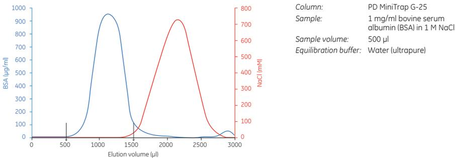
Fig 2.12. Removal of NaCl from BSA using the gravity protocol. The protein recovery was 95%.
