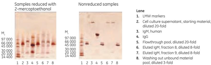
**Fig 3.29.** SDS-PAGE on PhastSystem using PhastGel 4–15, silver staining.
