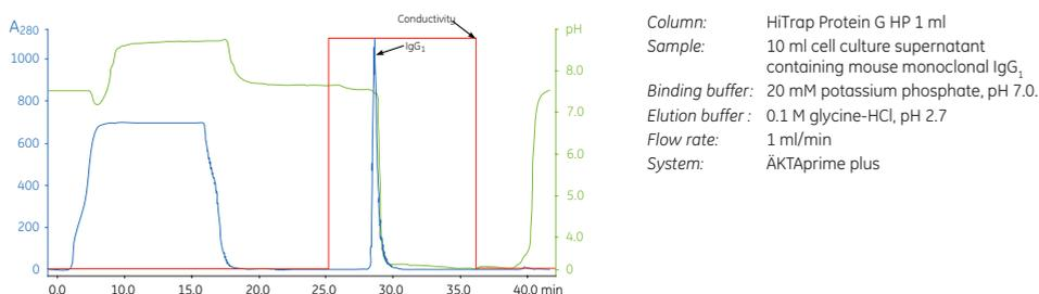
**Fig 6.5.** Capture step in a two-step purification of mouse monoclonal IgG<sub>1</sub> using HiTrap Protein G HP. The curves shown are absorbance (blue), pH (green), and conductivity (red).
