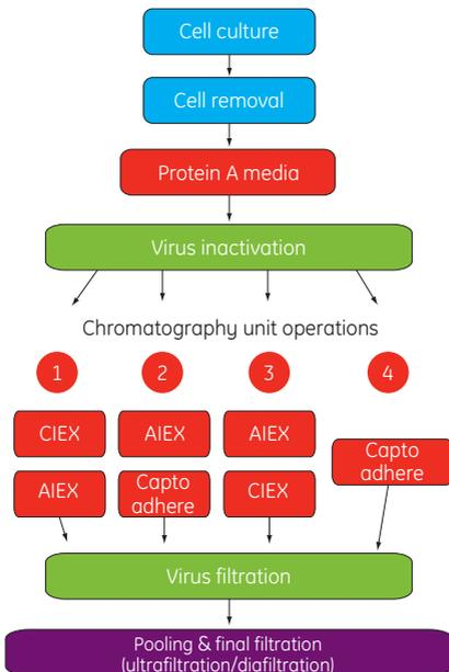
**Fig 7.1.** Overview of different combinations of chromatography unit operations in a MAB purification process.
