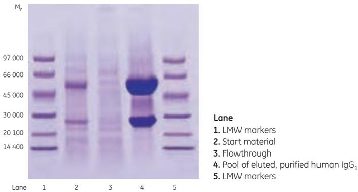
**Fig 3.25.** (A) Purification of human IgG<sub>1</sub> in one step on HiTrap MabSelect Xtra 1 ml on ÄKTAexplorer™ 10. (B) SDS-PAGE analysis on ExcelGel SDS Gradient 8-18, reducing conditions.
