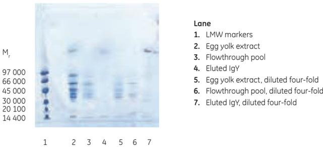
**Fig 3.31.** SDS-PAGE of nonreduced samples on PhastSystem using PhastGel 4-15, Coomassie staining.
