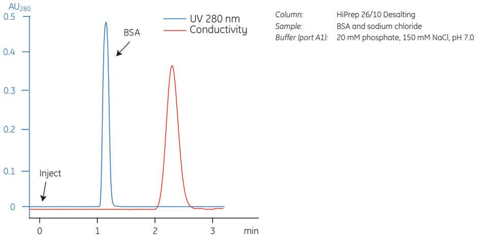
Fig 2.7. A typical desalting of BSA using a chromatography system.
