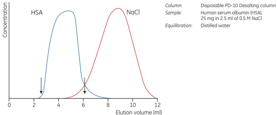
**Fig 2.14.** Removal of NaCl from albumin solution. A PD-10 Desalting column was equilibrated with distilled water. The sample contained human serum albumin (25 mg) dissolved in 2.5 ml of 0.5 M NaCl solution. A total of 23.8 mg albumin was recovered in 3.5 ml eluent corresponding to a yield of 95.3% (between arrows). Initial total salt content of sample before desalting was 2%.
