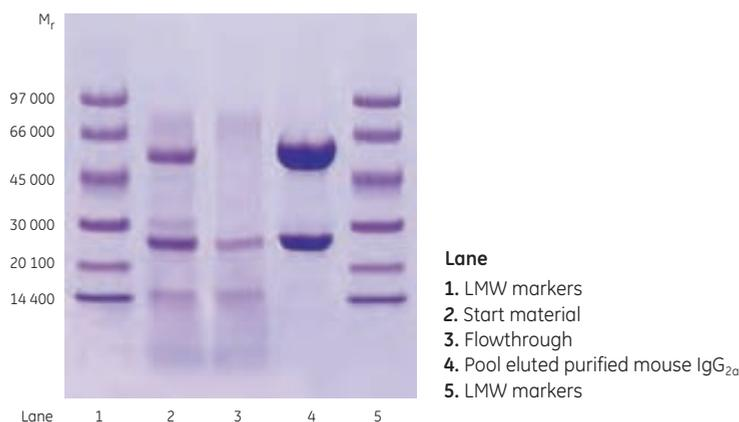
**Fig 3.24. (A)** Purification of IgG<sub>2a</sub> using HiTrap MabSelect 1 ml in an automated, two-step purification on ÄKTExpress™ MAB **(B)** SDS-PAGE analysis on ExcelGel SDS Gradient 8-18, reducing conditions.
