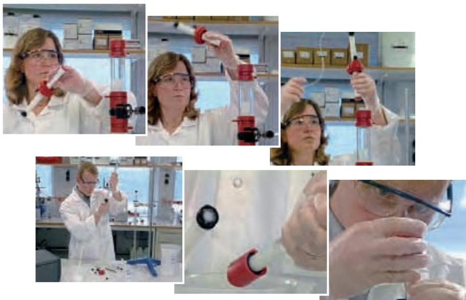
**Fig A5.1.** “Column Packing – The Movie” provides a step-by-step demonstration of column packing.
