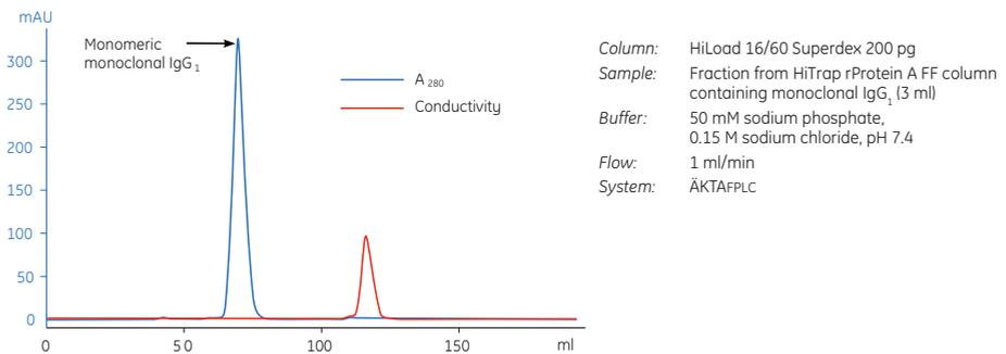
**Fig 6.3.** Polishing on HiLoad 16/60 Superdex 200 pg.
