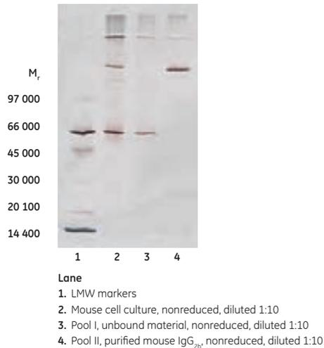
**Fig 3.21. (A)** Purification of mouse IgG<sub>2b</sub> from ascites on a 1 ml HiTrap rProtein A FF column using a syringe. **(B)** Analysis of eluted IgG<sub>2b</sub> by SDS-PAGE on PhastSystem and a PhastGel Gradient 10-15 precast gel revealed a purity of 95% (silver staining).
