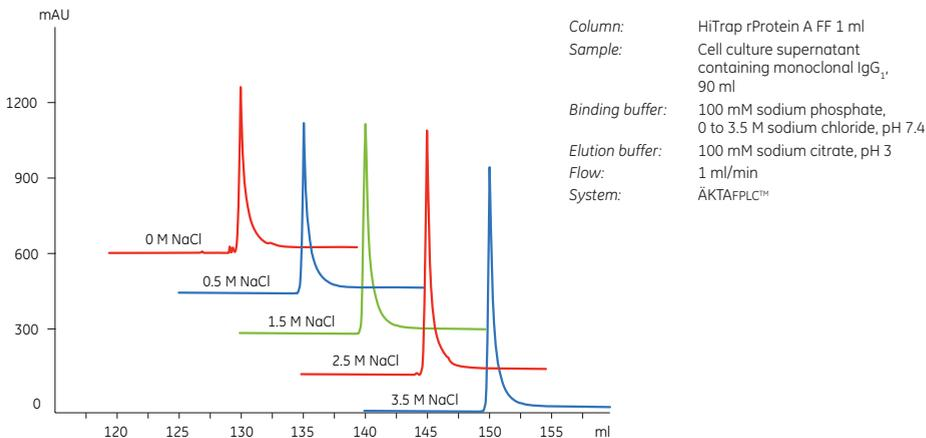
Fig 6.1. Automatic scouting of optimal salt concentration in the binding buffer on HiTrap rProtein A FF.
