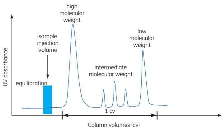
**Fig A9.7.** Typical GF elution.
