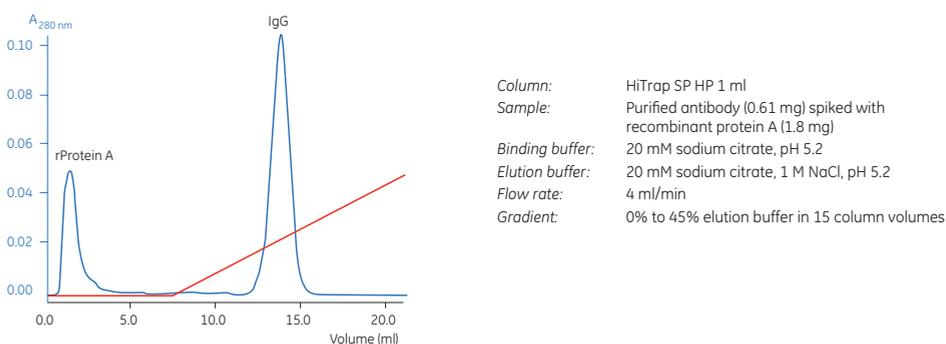
**Fig 4.5.** Removal of protein A from mouse IgG<sub>2b</sub> by cation exchange chromatography on HiTrap SP HP. Recombinant protein A was spiked into mouse IgG<sub>2b</sub> previously purified on rProtein A Sepharose Fast Flow.
