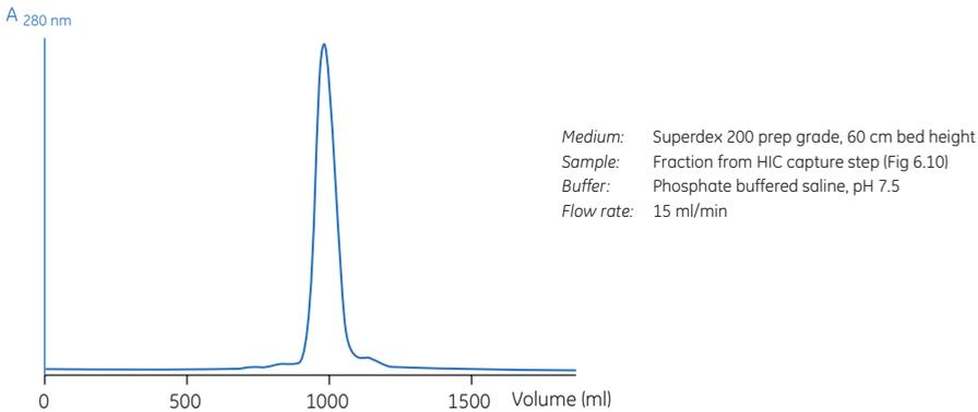
**Fig 6.11.** Polishing of mouse monoclonal IgG<sub>1</sub> anti-IgE using Superdex 200 prep grade.
