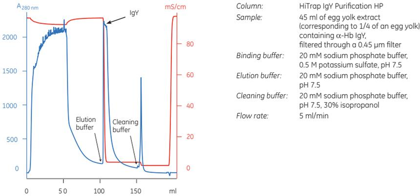
**Fig 3.30.** Purification of IgY on HiTrap IgY Purification HP.
