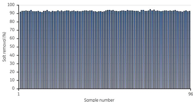
**Fig 2.10.** Removal of NaCl from BSA on a PD MultiTrap G-25 96-well plate showed highly reproducible results. The average desalting capacity was 93% and the well-to-well variation was 1% (relative standard deviation).
