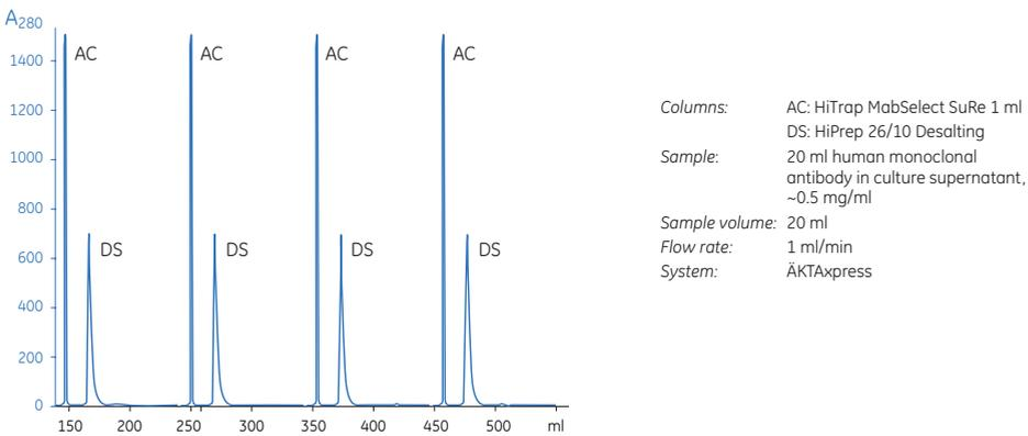
**Fig 6.8.** Chromatogram of four repetitive runs showing purification of human monoclonal antibody from cell culture by affinity chromatography (AC) and desalting (DS).
