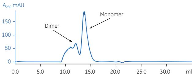
Fig 4.4. Separation of the monomer and dimer of a monoclonal antibody on Superdex 200 10/300 GL.
