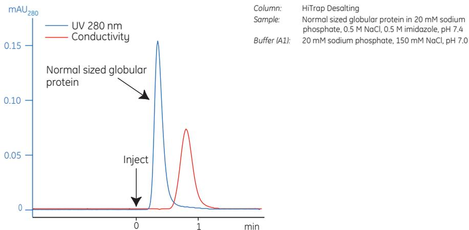
**Fig 2.5.** Typical desalting of a normal sized globular protein using a chromatography system.
