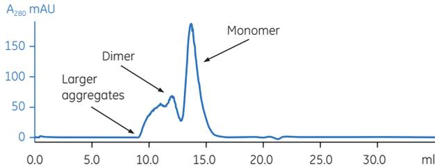
**Fig 3.2.** Gel filtration is a technique often used as a polishing step in antibody purification, as well as a method to remove dimeric, monomeric, and large aggregate forms of antibody. The chromatogram shows a separation of monomer, dimer, and larger aggregates of a monoclonal antibody using a prepacked Superdex 200 10/300 GL column.
