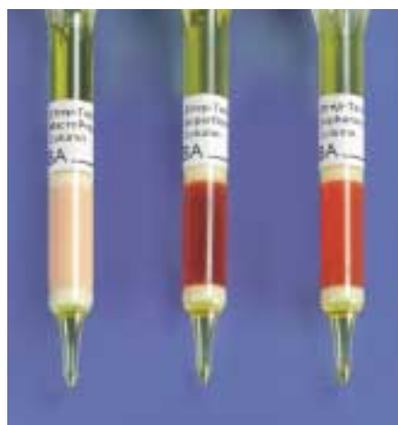
Strep-Tactin columns regenerated with HABA (see also pages 12, 17): Strep-Tactin MacroPrep, Superflow and Sepharose (left to right). Since MacroPrep is not as transparent as Sepharose or Superflow, the color shift to red is less visible. Scale: reduced.
