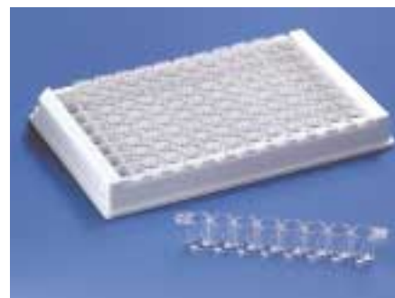
Microplate consisting of twelve 8-well strips coated with Strep-Tactin.
