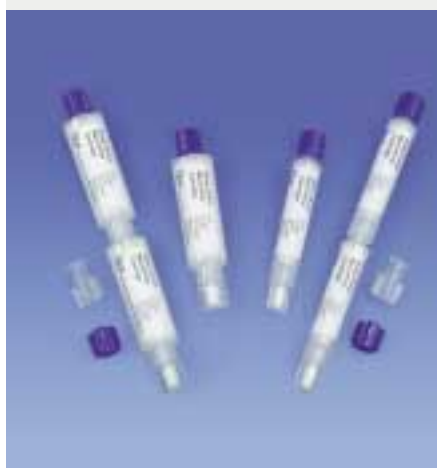
Cartridges with 1 ml or 5 ml Strep-Tactin Superflow® or Strep-Tactin MacroPrep® for low pressure chromatography (see pages 23, 24). Cartridges can be connected in series to enlarge capacity, and can be used with syringes. Adapters are available for use with peristaltic pump chromatography systems or FPLC/HPLC workstations (see table on the right). The cartridges have a female luer lock inlet and a male luer lock outlet. Also available with Ni-NTA resin (see pages 39, 40). Scale: reduced.
