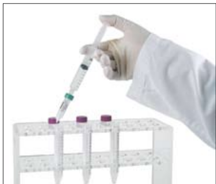
Fig. 6. Syringe purification using a Bio-Scale Mini Profinity eXact cartridge and poly column rack.
