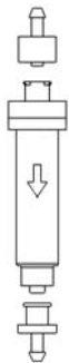
Fig. 3. Cartridge and fittings. Luer fittings and column: a cartridge should be mounted vertically with the arrow on the cartridge pointing downward.
