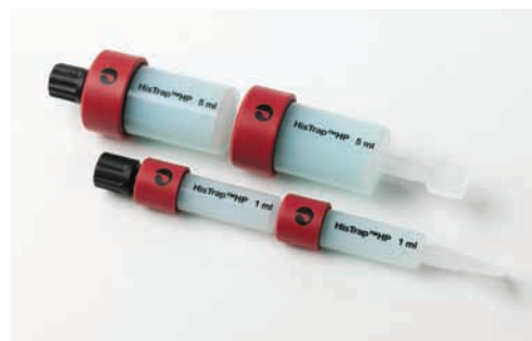
Fig 13. Quick and predictable scale-up by coupling two HisTrap HP 1 ml or 5 ml columns in series.
