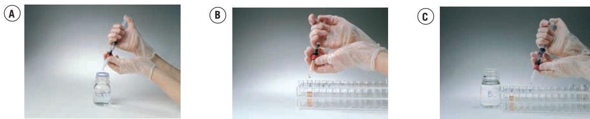
Fig 12. Using HisTrap HP 1 ml with a syringe. A) Prepare buffers and sample. Remove the column's top cap and twist-off the end. Wash and equilibrate. B) Load the sample and begin collecting fractions. C) Wash and elute, continue collecting fractions.
