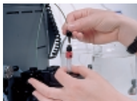
Connecting the column.
