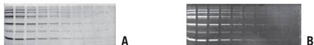
Fig 4. Images of an SDS-PAGE gel containing protein markers stained with Deep Purple and imaged (A) on a Typhoon 9410 imager with 532 nm laser and 560LP filter and (B) on the BioChem CCD-based imager with 365 nm UV transilluminator.
