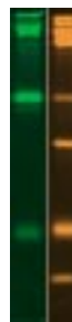
Figure 3. CandyCane glycoprotein molecular weight standards with four glycosylated and four nonglycosylated proteins. The standards were electrophoresed through two identical 13% polyacrylamide gels. Both lanes contain ~0.5 \mu g of protein in each band. The left lane is stained with Pro-Q Emerald 300 reagent. The right lane is stained with SYPRO Ruby protein gel stain (available in kit P-21855) to detect all eight marker proteins.
