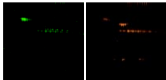
Figure 2. 2-D gel stained with SYPRO Ruby protein gel stain and Pro-Q Emerald reagent. Combined Cohn fractions II and III from cow plasma, containing primarily \beta - and \gamma -globulins, were run on a 2-D gel and stained first with Pro-Q Emerald 300 reagent (left) and then with SYPRO Ruby protein gel stain (right).
