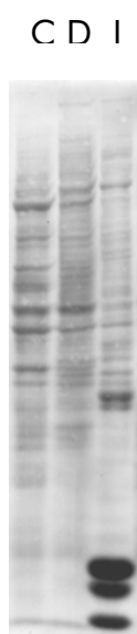
Figure 1 Fractions obtained after processing cell lysates using the Qproteome Nuclear Protein Kit. C: Cytosolic fraction; D: nucleic-acid-binding protein fraction; I: “Insoluble” fraction.
