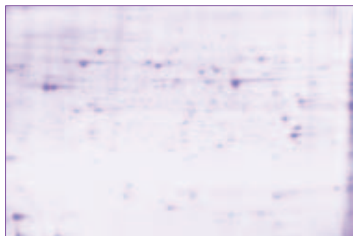
Figure 26. A GelCode™ Blue Stain Reagent-stained 2-D gel. The gel is an isolated hydrophilic fraction obtained using the Mem-PER® Kit (Product # 89826) from NIH3T3 cells run on a pH 5-8 IPG strip. Approximately 80 µg of protein was applied to the gel. The second dimension was performed on an 8-16% SDS-PAGE.
