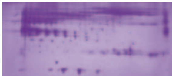
Figure 13. 2-D gel of human serum processed with the ProteoSeek™ Antibody-Based Albumin/IgG Removal Kit. Approximately 30 \mu g of processed human serum was isoelectric-focused on a pH 5-8 strip and then separated in the second dimension on an 8-16% SDS polyacrylamide gel. SilverSNAP® Stain II (Product # 24612) was used to visualize bands. With albumin and IgG removed, low-abundant proteins are readily identified.
