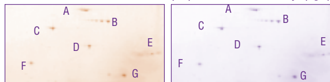
2-D Marker Shown Stained with Silver (left) and Coomassie Blue Dye (right)
