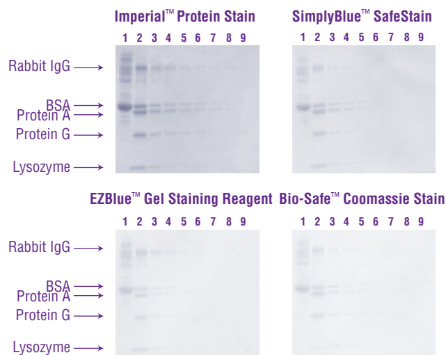
Figure 20. Imperial™ Protein Stain is fast and sensitive. Proteins were separated on Novex 4-20% Tris-glycine gels, stained for 5 minutes and destained 3 x 5 minutes in water. Lane 1: BSA only (6 µg), Lanes 2-9 contained the indicated proteins at the following concentrations: Lane 2: 1,000 ng, Lane 3: 200 ng, Lane 4: 100 ng, Lane 5: 50 ng, Lane 6: 25 ng, Lane 7: 12 ng, Lane 8: 6 ng and Lane 9: 3 ng.
