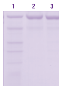
Figure 2. SDS-PAGE analysis of the inhibition of protease activity using Halt™ Protease Inhibitor Cocktails. Bovine serum albumin (BSA) was incubated overnight at 37°C in the presence of the protease papain. Lane 1 shows digestion of BSA in the absence of protease inhibitors. Lane 2 shows BSA digestion in the presence of Halt™ Protease Inhibitor Cocktail. Lane 3 shows BSA digestion in the presence of Halt™ Protease Inhibitor Cocktail, EDTA-Free.
