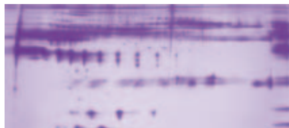
Figure 14. 2-D gel of human serum processed with ProteoSeek™ Albumin/IgG Removal Kit. Approximately 30 µg of processed human serum was isoelectric-focused on a pH 5-8 strip and then separated in the second dimension on an 8-16% SDS polyacrylamide gel. SilverSNAP® Stain II (Product # 24612) was used to visualize bands.
