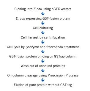
**Fig. 1.** General purification and on-column cleavage protocol for GST-fusion proteins.
