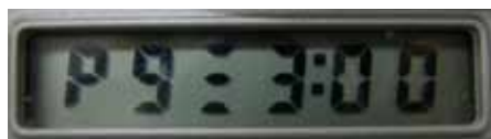
Figure 1. LCD display of the iBlot® Gel Transfer Device during operation of the P9 program. The P9 program has three substeps; the active substep is indicated on the display by the number of horizontal lines.
