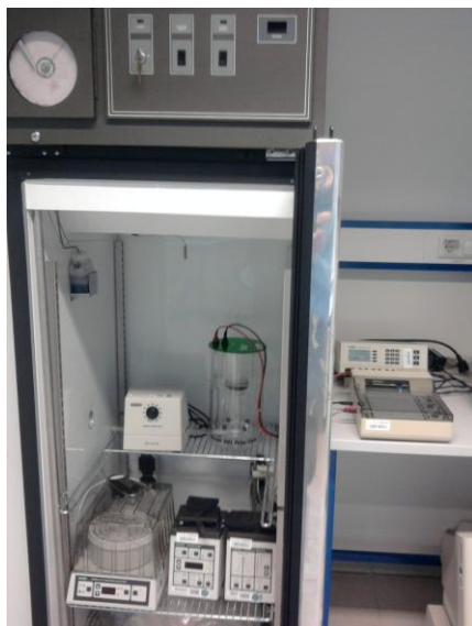
Fig. (1). Equipment for analytical electrophoresis: electrophoresis chamber, peristaltic pump, fraction collector, buffer recirculation pump and UV detector (in a refrigerator), power supply (5 W) and recorder (on a table).
