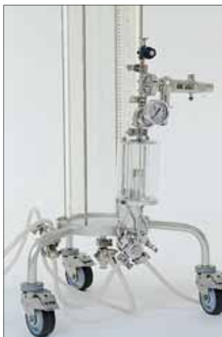
Air trap, top valve, manometer and safety valve.
