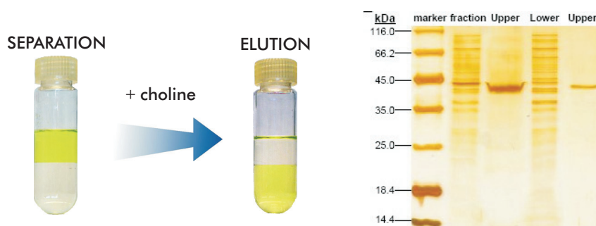
Figure 1. Purification of a GFP-LYTAG fusion protein expressed with the CASCADE™ system in the E. Coli host strain REG1. A 10 ml crude cell lysate was prepared from a 250 ml culture, and mixed with Top Lower Solutions. After separation of the two phases, addition of choline led to migration of the GFP-LYTAG fusion protein, from the upper to the lower phase.
