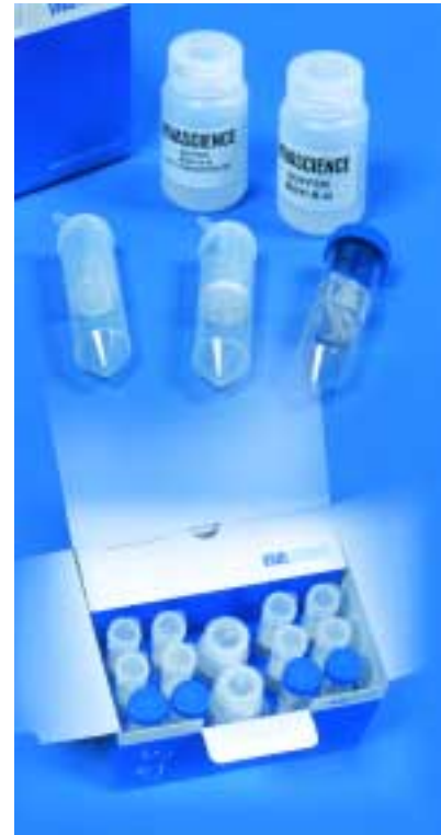
One Vivapure Q Maxi acidic spin column will bind approximately 60-80 mg of protein.
