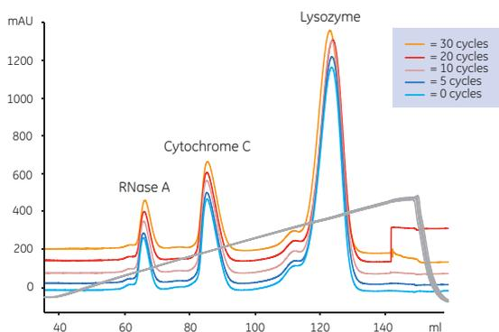
**Fig 4.** CIP study of MacroCap SP. The performance of MacroCap SP in the separation of RNase A, cytochrome C, and lysozyme was unaffected following 30 cycles of a CIP procedure. CIP conditions per cycle: 5 column volumes (CV)  $H_2O$ , 2 CV 0.5 M NaOH followed by 40 min static contact, 2 CV  $H_2O$ , 2 CV acidic solution ( $\sim$ pH 2) followed by 40 min static contact, 2 CV  $H_2O$ , 5 CV 0.5 M NaOH followed by 40 min static contact, and 5 CV  $H_2O$ .
