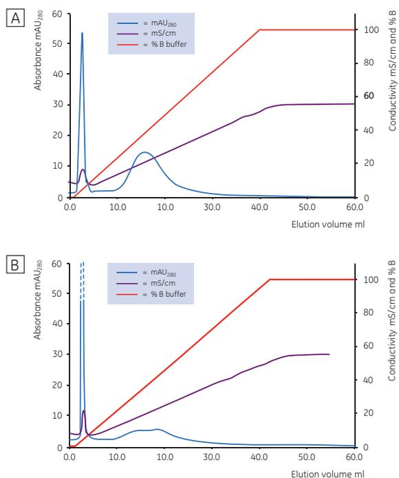
**Fig 3.** Binding and elution of a pure (96% by HPLC) sample of IgM ( $M_n = 750\,000$ ) (Sigma Aldrich, USA) on (A) MacroCap SP and (B) SP Sepharose High Performance. The large pore structure of MacroCap SP gives it a greater capability to bind large biomolecules.
