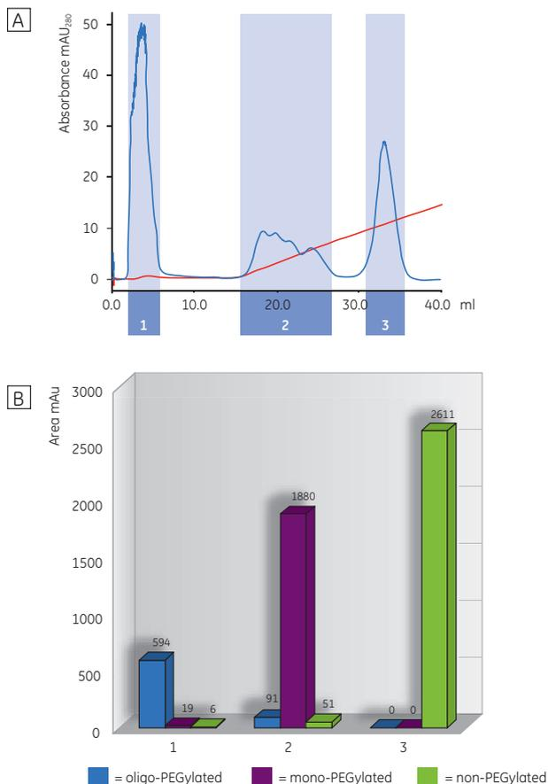
**Fig 2.** PEGylated cytochrome C<sup>1</sup> separated on MacroCap SP. **(A)** Chromatograms of the separation. Fractions that were pooled for the size exclusion chromatography (SEC) analysis are indicated in blue and numbered. **(B)** Pooled fractions indicated in **(A)** were analyzed by SEC on Superdex™ 200 for the amounts of oligo-, mono-, and non-PEGylated proteins.
