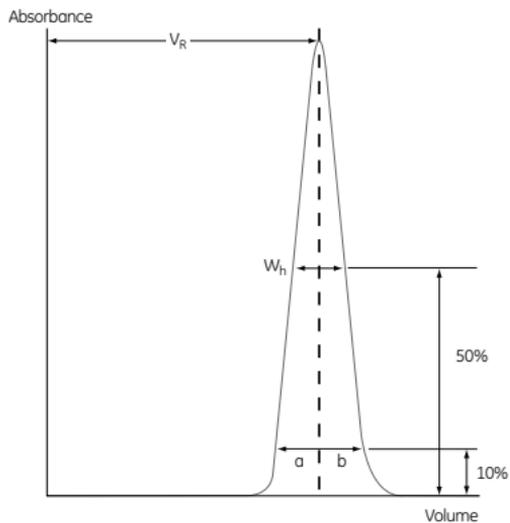
**Fig 11.** A typical test chromatogram showing the parameters used for HETP and  $A_s$  calculations.
