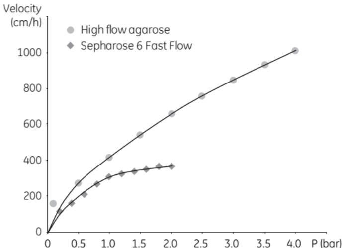
**Fig 2.** Pressure-flow properties for the high flow agarose base matrix used for Capto adhere compared to Sepharose™ 6 Fast Flow. Running conditions: BPG™ 300 (30 cm i.d.) open bed at settled bed height of 20 cm, with water at 20°C.
