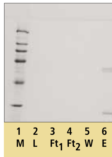
Figure 4. 500 column volumes [2,000 ml of dilute feedstock (2.7 mg IgG/l)] applied to a 3.9 ml column (1 x 5 cm). SDS-PAGE of Markers (M); 2: Load (L); 3: Flow through-1 (Ft1); 4: Flow through-2 (Ft2); 5: Wash (W); 6: Eluate (E).
