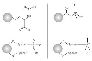
**Fig 3.16.** Design principles of CDM libraries. Multimodal cation exchangers (left) and multimodal anion exchangers (right) are illustrated.
