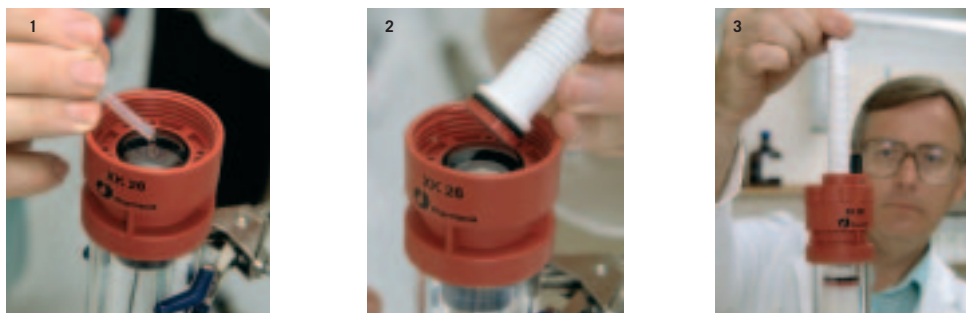
Fig. 70. Adding the top adaptor.
