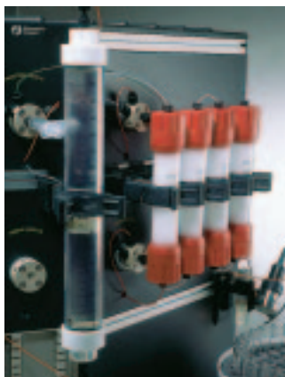
Fig. 51. Four HiPrep 26/10 Desalting columns connected in series.
