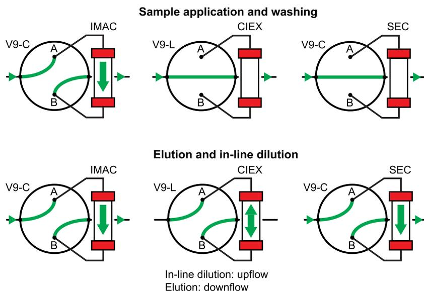
**Fig. 4.** Fluidic path and valve positions during automated three-column purification of  $t\beta 1$ -AR. Sample loading and washing on IMAC column is achieved in downflow direction. During in-line dilution sample from IMAC is stored in upflow direction on CIEX and further eluted in downflow direction on SEC.
