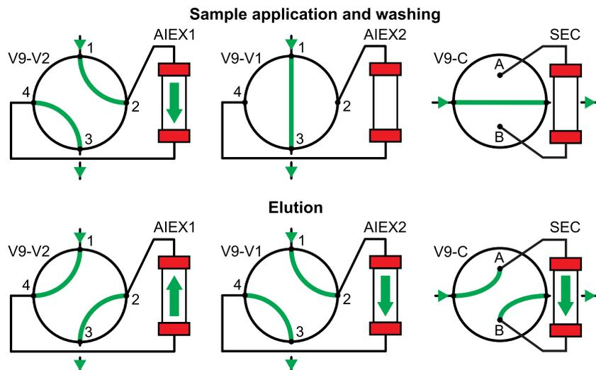
**Fig. 2.** Fluidic path and valve positions during automated three-column purification of GFP. Sample loading and washing on AIEX column is achieved in downflow direction. During elution, AIEX1 is switched to upflow and AIEX2 and SEC to downflow direction.
