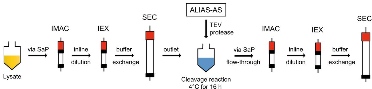
**Fig. 7.** Example of purification scheme involving enzymatic reactions. The His-tagged protein of interest is initially purified using an IMAC to IEX to SEC scheme. ALIAS-AS is used to inject TEV protease into an external vessel, where the cleavage reaction takes place. After cleavage, the reaction solution is re-injected into the ÄKTA system and further polished using a second set of IMAC to IEX to SEC. An in-line dilution protocol is implemented between IMAC and IEX column transfers.
