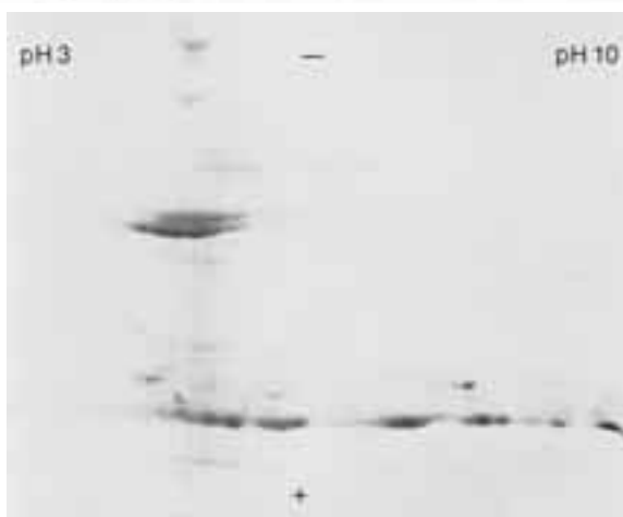
Fig. 23. IEF followed by SDS-gradient polyacrylamide gel electrophoresis of potato proteins. First dimension: Isoelectrofocusing for 20 h at 500 V in a gradient of Pharmalyte pH 3–10 in a 5 % polyacrylamide rod (150 mm \times 2.7 mm). Second dimension: Electrophoresis in a gradient (10–20 %) of polyacrylamide in 0.2 % SDS. Sample size: 100 \mu l.
