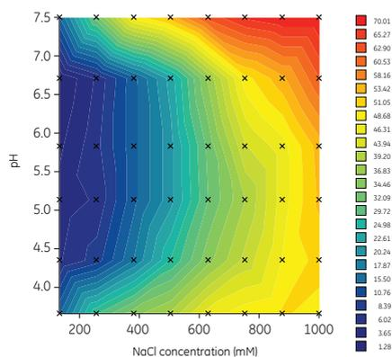
**Fig 4.42.** Pro-insulin yield (%) (first elution fraction) on Capto MMC as a function of NaCl concentration (150 to 1000 mM) and buffer pH (4 to 7.5). Assist software was used in obtaining these data.
