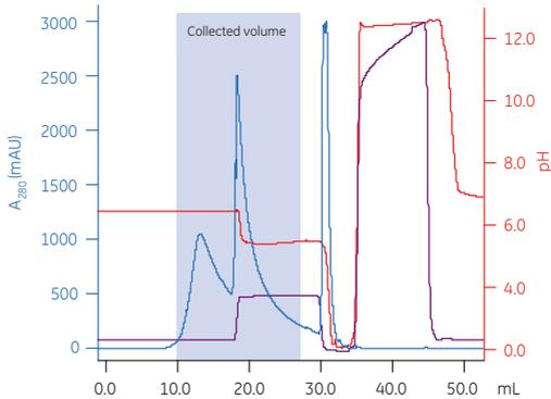
**Fig 4.24.** Chromatogram from the column verification. Blue: Absorbance at 280 nm. Red: pH. Purple: Conductivity (mS/cm).
