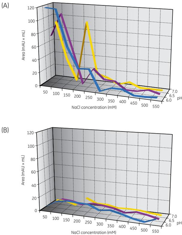
**Fig 4.19.** (A) Monomer and (B) aggregate elution profiles based on the data from PreDictor plates.
