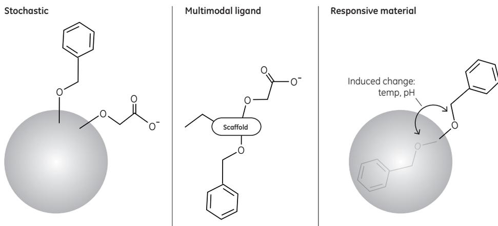
**Fig 2.1.** Schematics showing examples of creating a multimodal medium or column based on the three types of preparation methods described above.
