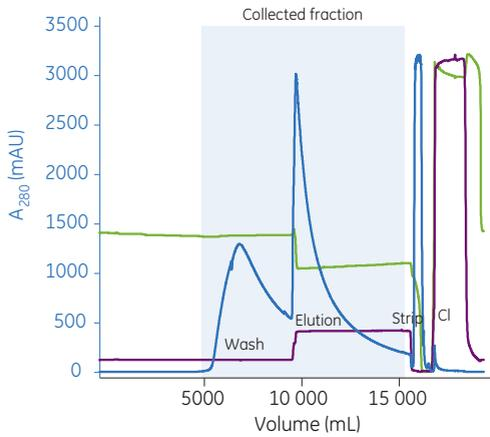
**Fig 4.27.** Chromatogram from the Capto adhere step.  $A_{280}$  trace is shown in blue, pH in green, and conductivity in purple.
