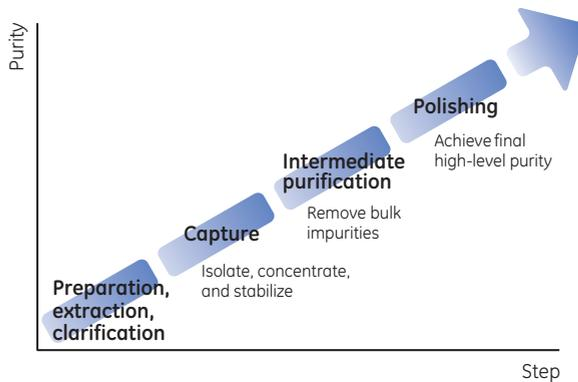
Fig 1.1. Illustration of the different stages in a purification process.
