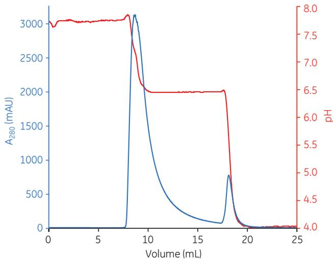
Fig 4.38. Step elution of MAb B using Capto adhere ImpRes.
