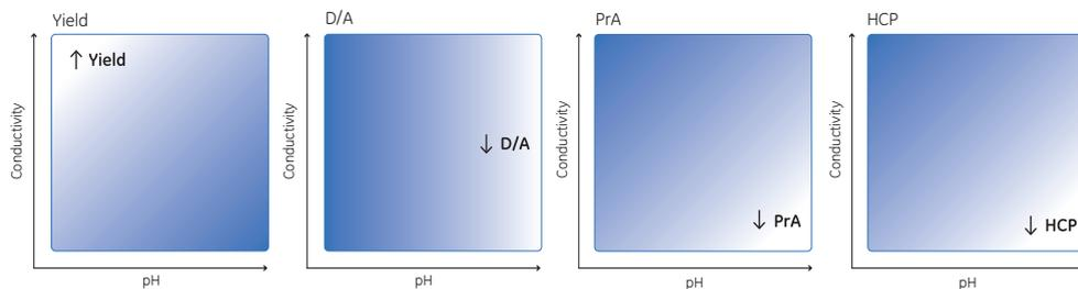
Fig 4.12. General trends with respect to loading conditions for yield, D/A, and Protein A and HCP clearance.
