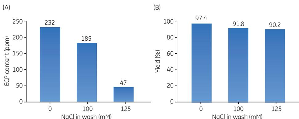
**Fig 4.59.** Purification of a recombinant DAb using Capto MMC ImpRes. (A) ECP contaminants in the elution pool and (B) DAb yield using different NaCl concentrations in the binding and wash buffers.
