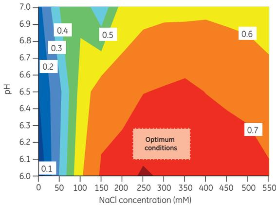
**Fig 4.20.** Effect of NaCl concentration and buffer pH on a normalized objective function purity  $\times$  yield (shown in labels within image).
