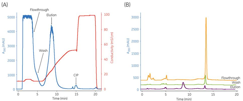
**Fig 4.44.** (A) A 2 mL crude sample, pH 5.2 in 8 M urea, loaded on a Tricorn 1 mL column packed with Capto MMC and eluted with a linear combined salt and pH gradient from 150 to 1000 mM NaCl and pH 5.2 to 7.5 for 7 CV. (B) Corresponding Mono Q analysis of the flowthrough, wash, and pooled fractions in the main elution peak. In both A) and B), detection was at 280 nm.
