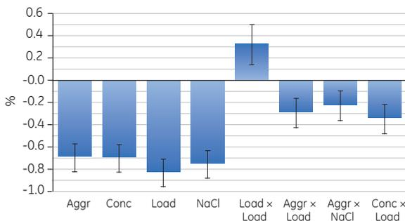
**Fig 4.21.** Coefficients plot for monomer purity.
