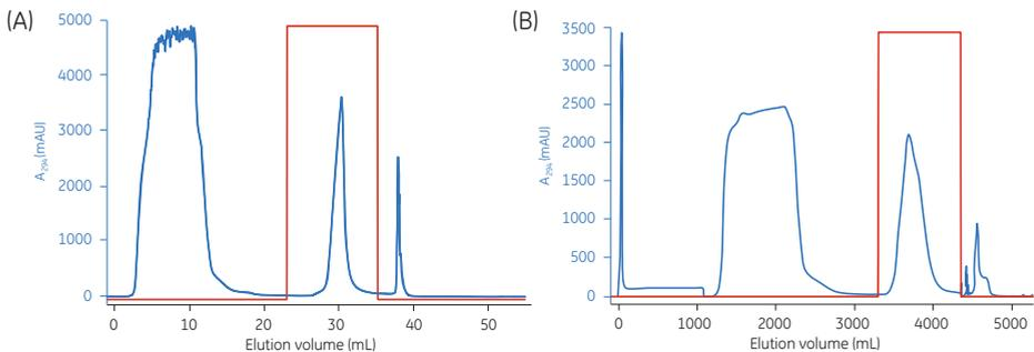
**Fig 4.48.** Straightforward scale-up from A) Tricorn 5/100 to B) AxiChrom 50 (100 times). In both cases the purification factor was 4 and the recovery was 93%.
