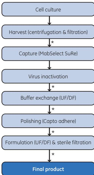
**Fig 4.26.** Flow scheme of the purification process in which steps involving in-process filtration of the sample to reduce bioburden are indicated with asterisks (\*). UF/DF = ultrafiltration/diafiltration.
