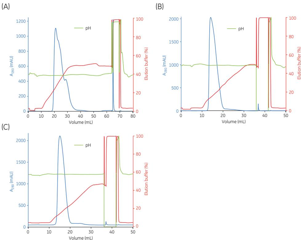
**Fig 4.53.** Elution of the MAb in a salt gradient at three different pH: (A) pH 5.0, (B) pH 6.0, and (C) pH 7.0.
