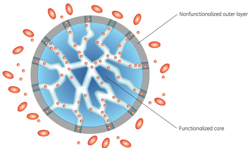
**Fig 3.14.** Schematic cross-sectional view of a Capto Core 700 particle with an average diameter of 85  $\mu\text{m}$ . Small protein impurities can enter the interior of the matrix particle and bind to the ligand. Large molecular entities such as virus particles are hindered from entering the matrix.
