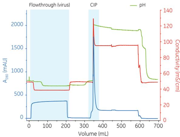
**Fig 4.61.** Two-step purification of influenza A/H1N1 virus after MF. After capture of the virus, final purification was achieved using Capto Core 700.
