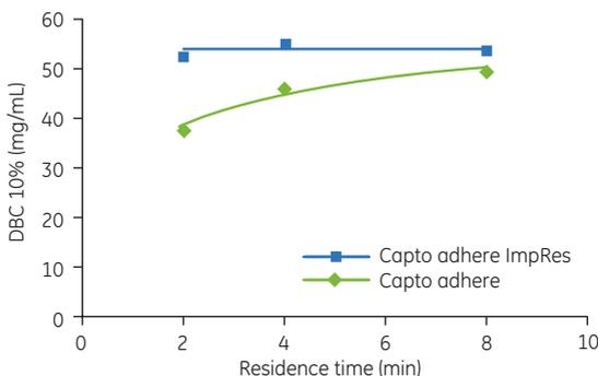
**Fig 3.6.** DBC of a MAB vs residence time. DBC at 10% breakthrough measured in 90 mM sodium phosphate, pH 7.75.
