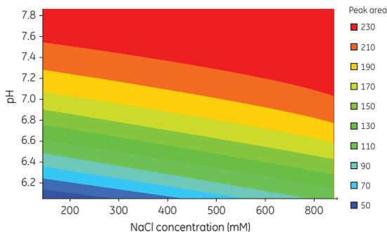
**Fig 4.45.** Response surface for the elution peak area of pro-insulin as a function of pH and NaCl concentration in mM. R<sup>2</sup> (explained variation) = 0.989, Q<sup>2</sup> (predicted variation) = 0.736. ÄKTA avant was used in obtaining these data.
