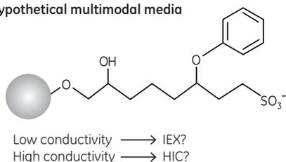
**Fig 2.4.** Multimodal media and chromatographic use. A combination of interaction modes can be expected with multimodal media. The type of interaction(s) will depend on conditions and characteristics of the target molecule. Int = interactions.
