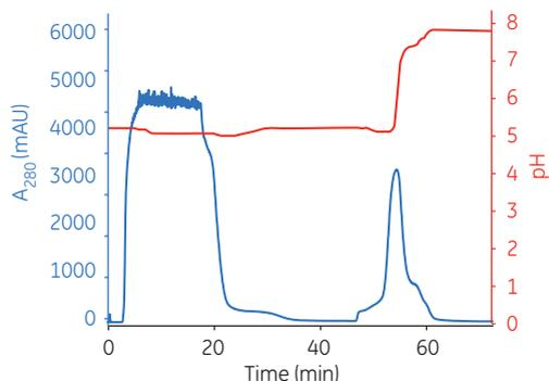
**Fig 4.47.** Chromatogram from the final (AxiChrom column) step after preceding columns. The pro-insulin crude sample was loaded on Capto MMC at pH 5.2 and 150 mM NaCl in a HiScreen (9 mL), HiScale (40 mL), and AxiChrom 50/300 (bed height 19.5 cm; 400 mL) column. An ÄKTA avant 150 system was used with the AxiChrom column.
