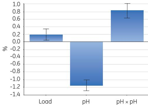
Fig 4.8. Coefficient plot for the D/A clearance model.
