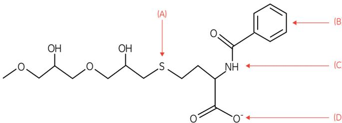
**Fig 3.8.** Capto MMC ligand. Interactions are shown by arrows: (A) for thiophilic; (B) for hydrophobic; (C) for hydrogen bonding; and (D) for electrostatic interactions.
