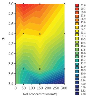
**Fig 4.40.** Response surfaces generated by Assist software for pro-insulin binding (g/L) as a function of NaCl concentration (x-axis) and buffer pH (y-axis) for SP Sepharose Fast Flow, Capto S, and Capto MMC, respectively. The range of binding capacities achieved is shown to the right of each surface. Black crosses represent actual data between results that have been interpolated.
