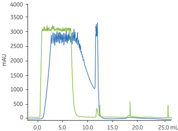
**Fig 4.2.** Establishing suitable conditions for DoE on Cpto adhere in flowthrough mode. Comparison of chromatograms obtained at different pH: pH 8.0 (blue curve) and pH 6.0 (green curve).
