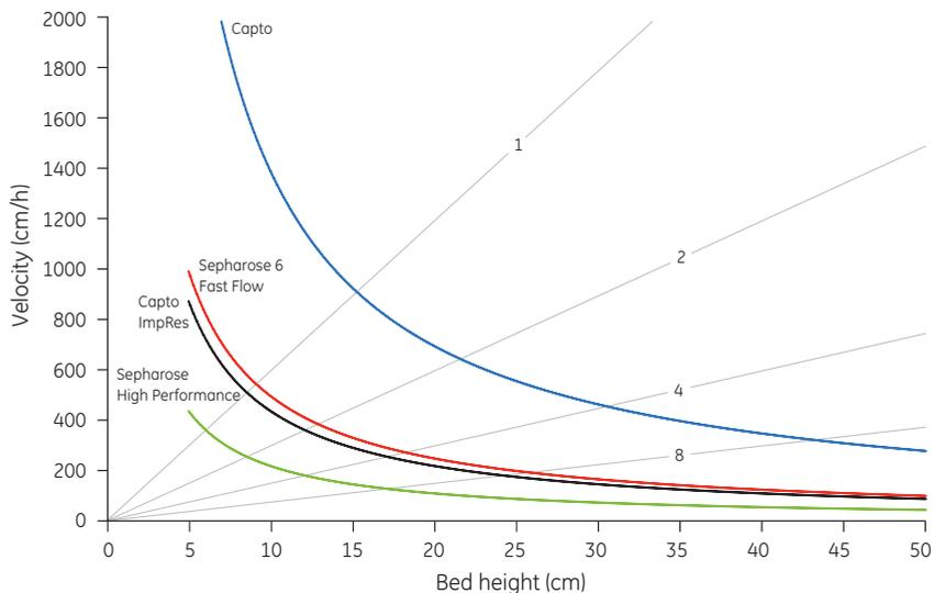
**Fig 3.1.** Comparison of the window of operation (area below the curves) at large scale for different base matrices. Gray lines give the residence time in the column in minutes. The particle size of Capto MMC/adhere is 75  $\mu\text{m}$ , and of Capto MMC/adhere ImpRes it is 40  $\mu\text{m}$ . See Appendix 1 for characteristics of the various multimodal media from GE Healthcare.
