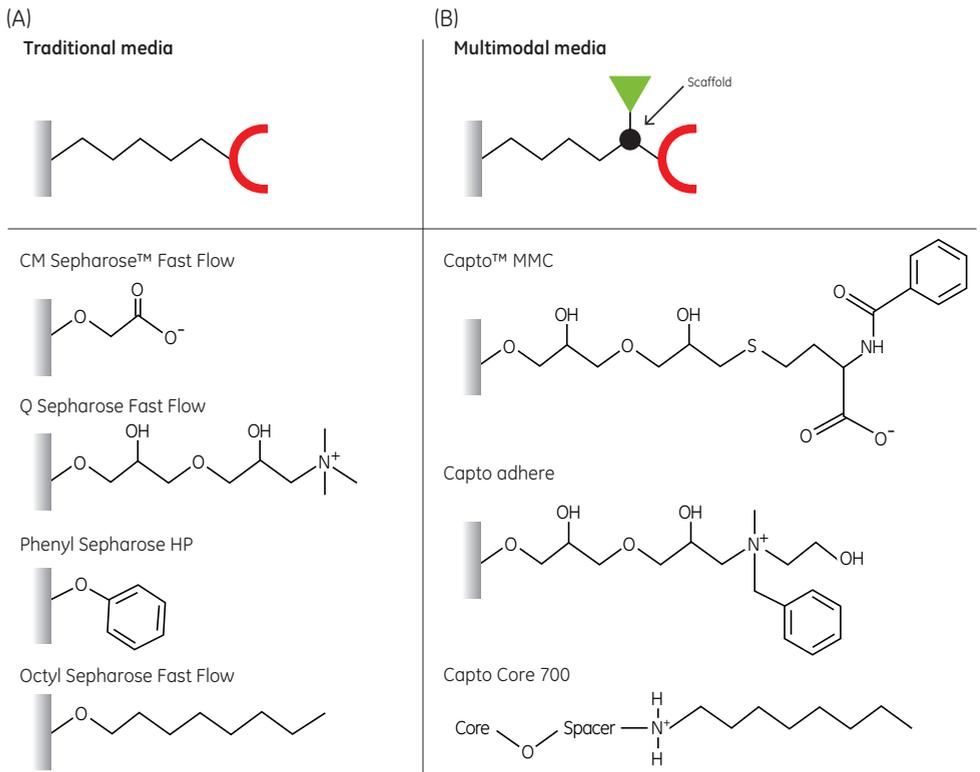
**Fig 2.3.** Comparison of traditional and multimodal media. (A) Schematic of traditional media and examples (CM Sepharose Fast Flow, Q Sepharose Fast Flow, Phenyl Sepharose HP, and Octyl Sepharose Fast Flow). (B) Multimodal media. Capto MMC, Capto adhere, and Capto Core are shown as examples. Note that the Capto Core 700 ligand is found only in the core of the bead.
