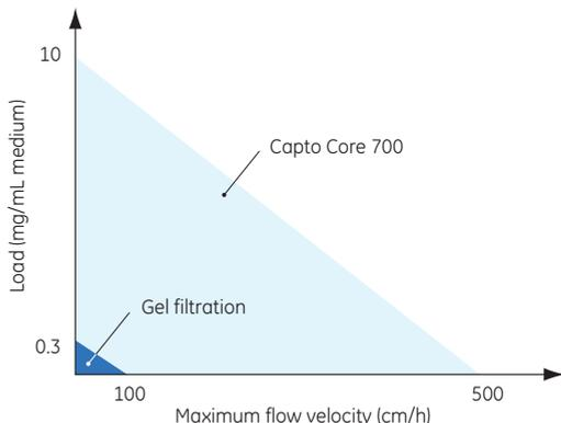
**Fig 3.15.** Schematic illustration of the significantly greater sample load and flow velocity enabled with Capto Core 700 in comparison with conventional GF media. Note that the schematic is not to scale.
