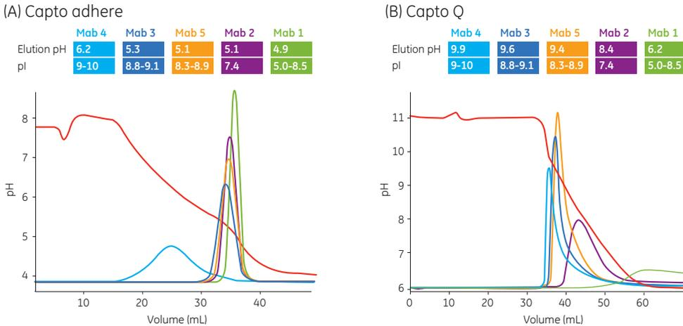
**Fig 3.3.** Different selectivity of Capto adhere compared with traditional ion exchangers. pH gradient elution of five MAbs on Capto adhere and Capto Q. For the pH gradient (A) A-buffer (equilibration buffer) was 20 mM Na-citrate + 20 mM Na-phosphate, pH 7.8, and B-buffer was buffer A at pH 4.0. (B) A-buffer was 20 mM Na-phosphate, 20 mM Tris, 20 mM glycine, pH 11, and B-buffer was buffer A at pH 6.2 Gradient: 0 to 100%B, 10 column volumes (CV).
