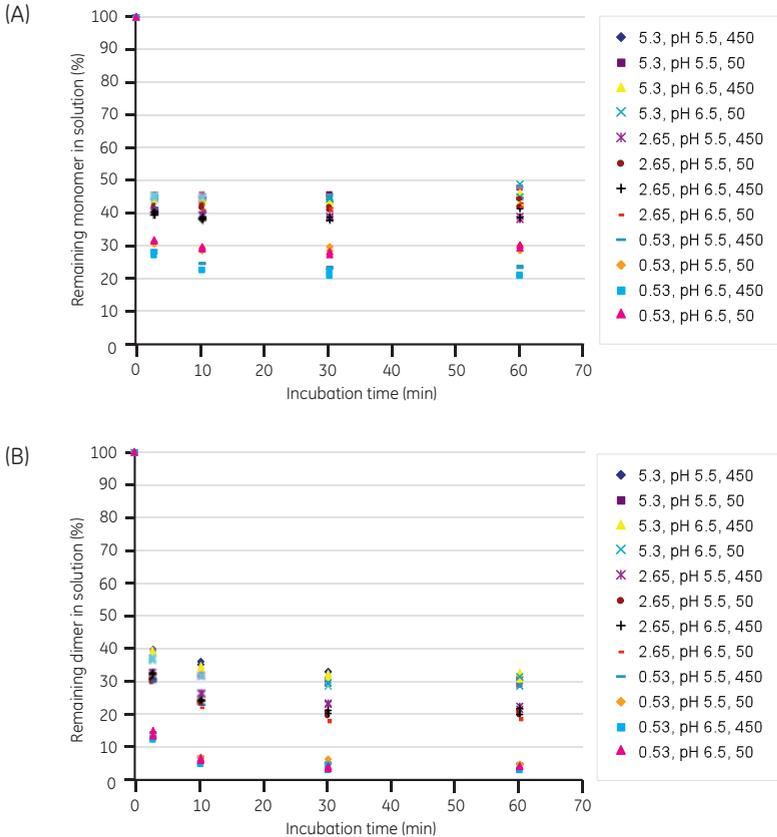
**Fig 4.16.** Adsorption curves of (A) monomer and (B) aggregates. This shows the remaining monomer and aggregate concentrations in the flowthrough fractions under the investigated conditions of antibody amounts, NaCl concentrations, and pH. Legends correspond to protein concentration (mg/mL), pH, and NaCl concentration (mM).
