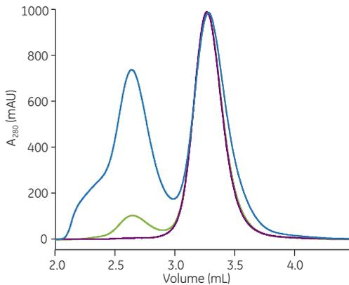
**Fig 4.28.** GF analysis of the MAb in the Capto adhere step—sample before purification (green), purified fraction (purple), and strip fraction (blue). The curves were normalized with respect to the monomer peak of the purified fraction.
