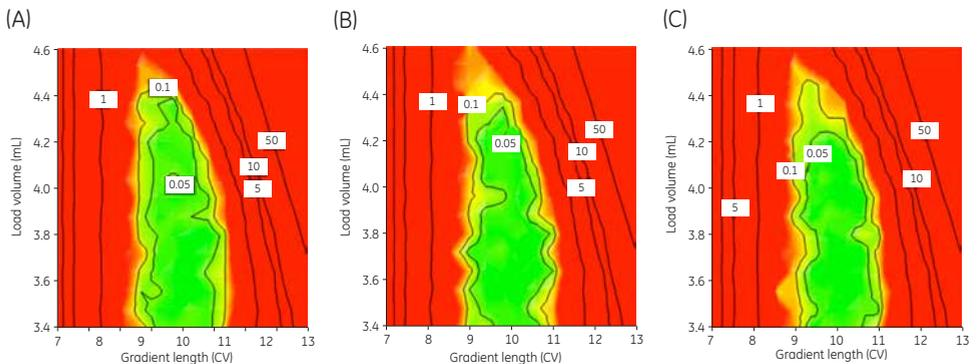
**Fig 4.56.** Contour plots from the Monte Carlo analysis showing risk of failing to meet the set criteria for aggregate level and pool volume in percentage, at flow velocities of (A) 46, (B) 49, and (C) 52 cm/h.
