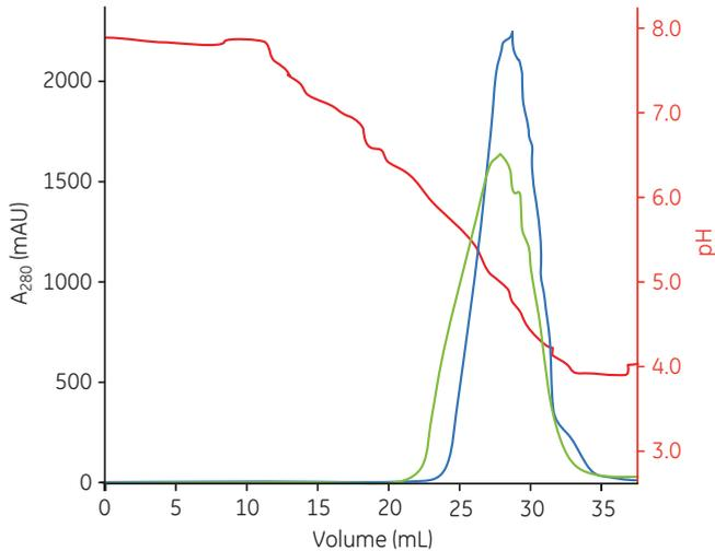
**Fig 4.33.** Gradient elution on Capto adhere ImpRes using elution buffer with NaCl (green curve) and without NaCl (blue curve) of MAb A, which was partially purified by protein A affinity chromatography.
