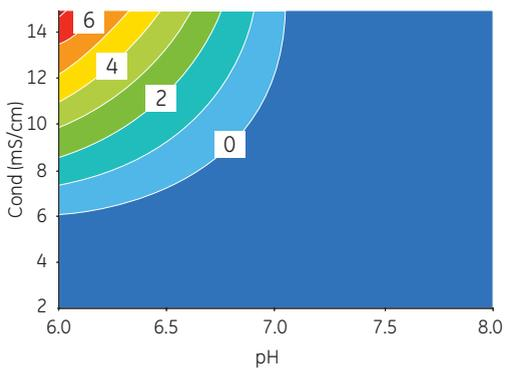
**Fig 4.7.** Response surfaces for the Protein A clearance model, conductivity versus pH. Protein A concentration expressed in ppm.
