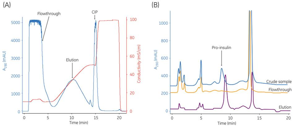
**Fig 4.43.** (A) A 2 mL crude sample, pH 5.2 in 8 M urea, loaded on a Tricorn 1 mL 5/50 column packed with Capto MMC and eluted by a linear salt gradient from 150 to 1000 mM NaCl for 7 CV. (B) Corresponding Mono Q analysis of crude sample, flowthrough, and one elution fraction (collected at the main elution peak maximum). In both A) and B), detection was at 280 nm.
