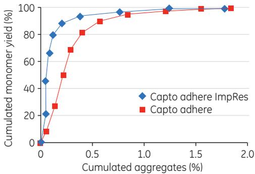
**Fig 4.37.** Cumulated aggregates vs cumulated MAb monomer yield after gradient elution using Capto adhere ImpRes and Capto adhere.
