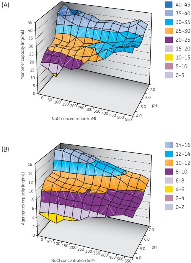
**Fig 4.17.** (A) Monomer and (B) aggregate capacities determined from the PreDictor plate experiments.
