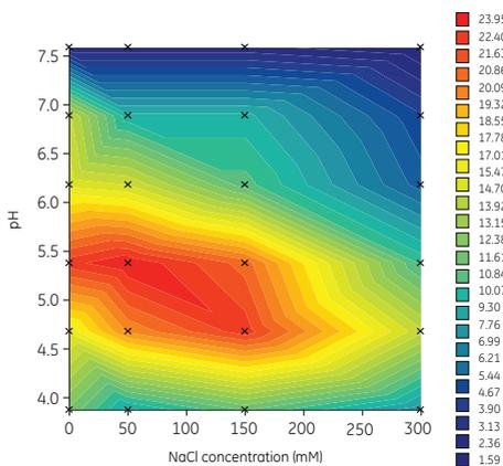
**Fig 4.41.** Response surface for binding (g/L) of pro-insulin on Capto MMC as a function of NaCl concentration (0 to 300 mM) and buffer pH (4 to 7.5). Assist software was used in visualizing this data.
