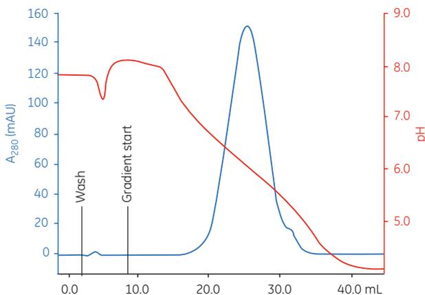
**Fig 4.1.** Establishing suitable conditions for DoE on Capto adhere in binding mode.
