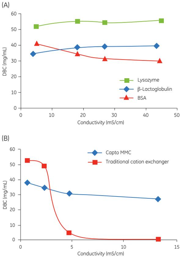
**Fig 3.9.** (A) DBC of Capto MMC at 1 min residence time for three different proteins at different conductivities. (B) Capto MMC allows a much larger operating range in terms of conductivity of the starting material than traditional cation exchangers.
