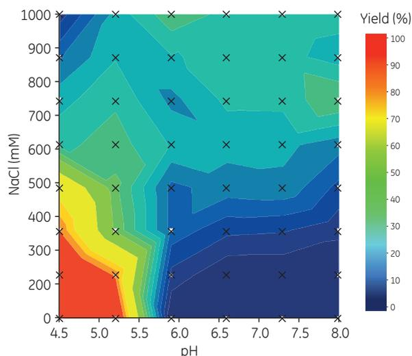
**Fig 4.32.** Screening of elution conditions in PreDicator plate. Yield obtained by varying elution pH between 4.5 and 8.0 and NaCl concentration between 0 and 1 M. Evaluation performed by Assist software for PreDicator plates.
