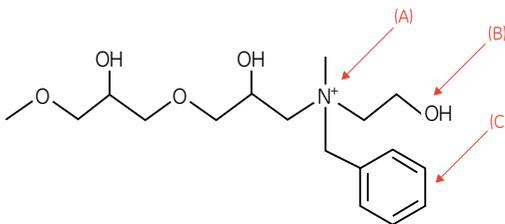
**Fig 3.2.** The design of the Capto adhere ligand, N-benzyl-N-methyl ethanolamine. This ligand exhibits several possibilities for interaction with proteins. The most pronounced are electrostatic interaction, hydrogen bonding, and hydrophobic interaction, as shown by arrows: (A) for electrostatic interactions; (B) for hydrogen bonding; and (C) for hydrophobic interactions.
