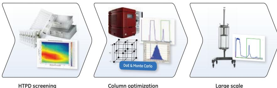
**Fig 1.3.** A typical workflow. Initial screening is performed in a high-throughput format, followed by optimization using a small column and verification in large scale. A discussion of Design of Experiments (DoE) and Monte Carlo simulations is provided in the text below.
