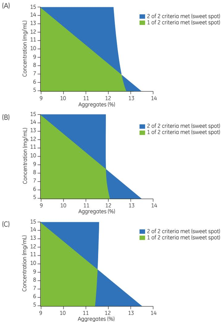
**Fig 4.23.** A sweet spot plot for IgG monomer yield and purity. The conditions for these plots were a sample load of 60 mg/mL media and elution with 300 mM of NaCl at the three different pH levels of: (A) 6.1; (B) 6.3; and (C) 6.5.
