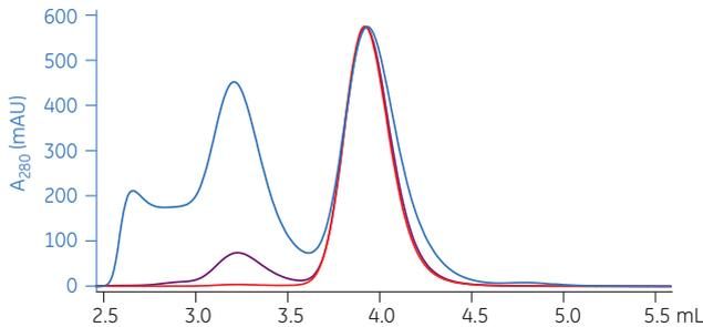
**Fig 4.25.** GF analysis of the start material (purple), flowthrough/elution fraction (red), and strip fraction (blue). All the curves were normalized against the flowthrough/elution fraction.
