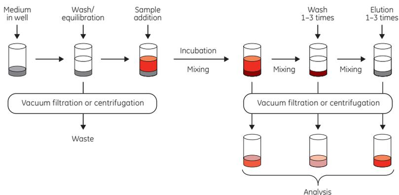
**Fig 4.39.** Schematic illustration of the workflow of a batch experiment in the wells of a PreDictor plate. The same steps would be employed in a column experiment, that is, equilibration, sample addition, wash, and elution. The gray color in the wells represents the chromatography medium; red shades (red and pink) represent different concentrations of protein solution. Brown represents the medium with bound sample.
