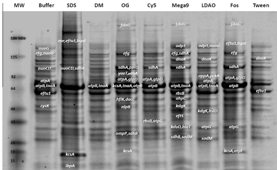
**Fig. 3.** Constitutive membrane proteins extracted by various detergents from the total cell membrane of *E. coli* XL-1 cells. Each detergent extract was concentrated to load an equal amount of protein (~50 µg) in each gel lane. The annotated proteins were each identified by peptide mass fingerprinting and, in some cases, further confirmed by MS/MS fragmentation.
