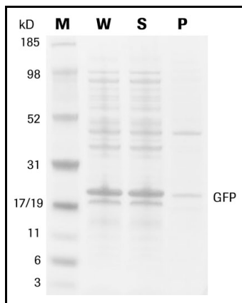
Fig. 1: SDS-PAGE analysis and Coomassie blue staining of proteins extracted from E. coli BL21 DE3 cells overexpressing GFP.
