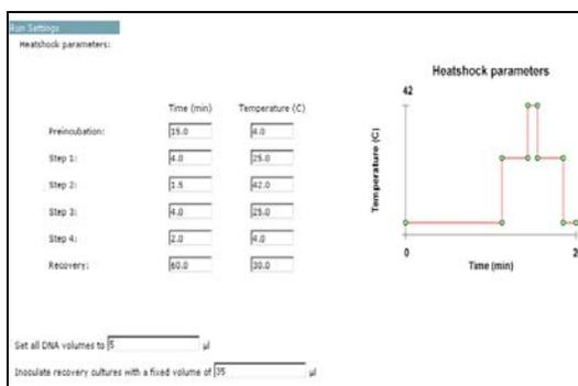
Set-up screen from the NextGen Sciences' orchestratorIMS software that controls the robotics systems
